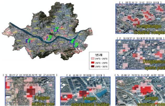
Figure 10. Surface temperature change analysis using ASTER TIR satellite image
