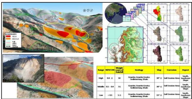
Figure 7. Mapping potential landslide hazard area
